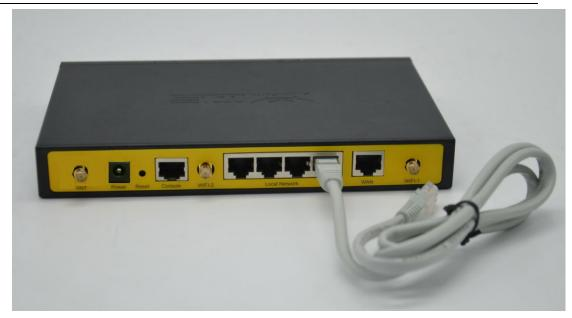
Insert the RJ45 end of the console cable into the RJ45 outlet with sign "console", and insert the DB9F end of the console cable into the RS232 serial interface of user's device.
