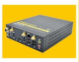
F4931-R2H is a low-power industrial computer independently developed by Four-Faith. It combines wireless cellular network and routing technology with industrial computer technology.
