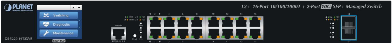
Figure 2-1-4: Front Panel of GS-5220-16T2XVR
