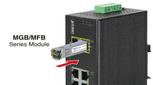
Figure 3-1: Plug-in the SFP Transceiver
