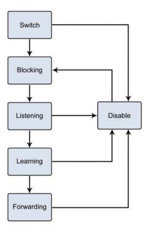
Figure 4-3-4-1: STP Port State Transitions
