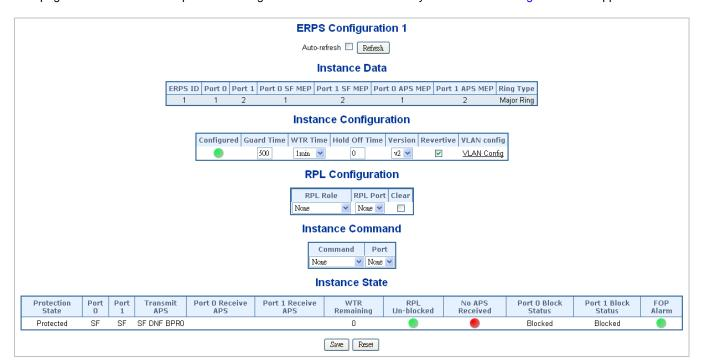
Figure 4-6-1-4: Ethernet Ring Protocol Switch Configuration page screenshot
