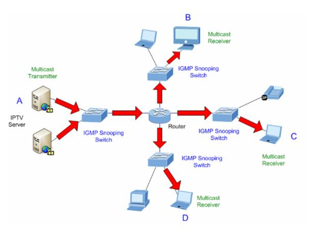
Figure 4-3-5-3: IGMP Snooping Multicast Stream Control
