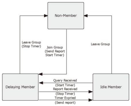
Figure 4-3-5-4: IGMP State Transitions
