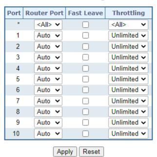
Figure 4-3-5-7: IGMP Snooping Configuration Page Screenshot
