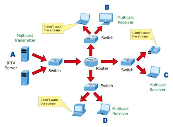
Figure 4-3-5-2: Multicast Flooding
