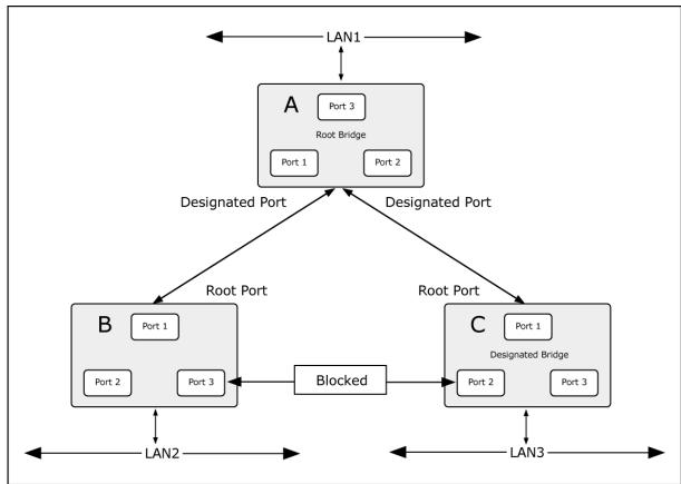
Figure 4-3-4-3: After Applying the STA Rules
