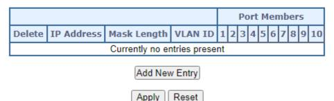
Figure 4-3-3-17: IP Subnet-based VLAN Membership Configuration page screenshot
