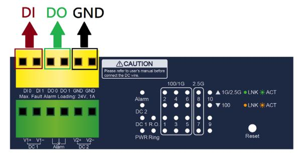
Figure 2-3: Wiring the Digital Input/Digital Output and Ground
