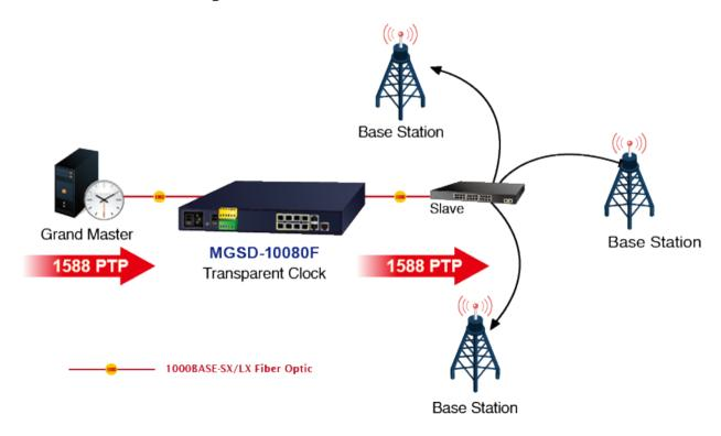
PTP was originally defined in the **IEEE 1588-2002** standard, officially entitled "Standard for a Precision Clock Synchronization Protocol for Networked Measurement and Control Systems" and published in 2002. In 2008 a revised standard, **IEEE 588-2008** was released. This new version, also known as PTP Version 2, improves accuracy, precision and robustness but is not backwards compatible with the original 2002 version.
