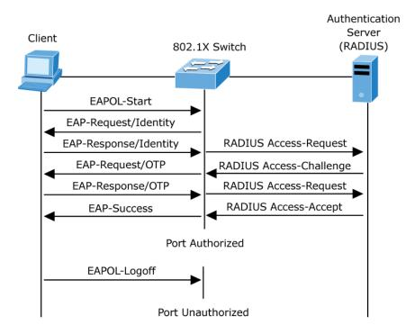
Figure 4-5-2-2: EAP Message Exchange
