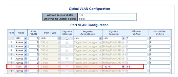
Figure 4-3-3-14: VLAN Overlap Port Setting & VLAN 1 - The Public Area Member Assign
