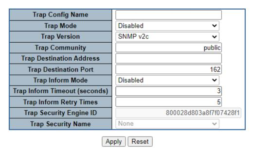
Figure 4-2-2-4: SNMP Trap Configuration Page Screenshot
