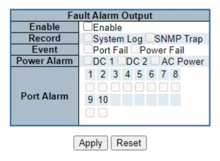
Figure 4-2-20: Fault Alarm Control Configuration page Screenshot
