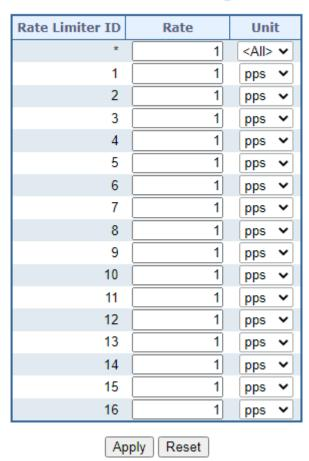
Figure 4-5-5: ACL Rate Limiter Configuration Page Screenshot
