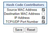
Figure 4-3-2-2: Aggregation Mode Configuration Page Screenshot
