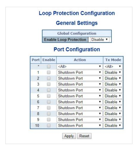
Figure 4-3-10-1: Loop Protection Configuration Page Screenshot
