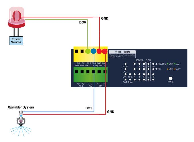
Figure 2-6: Wiring DO0 and DO1 to Open Detector
