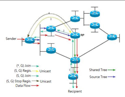
Figure 5-1 Join-in mechanism of PIM-SM
