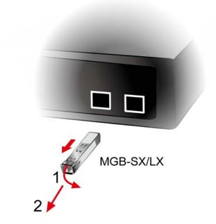
Figure 2-6: How to Pull Out the SFP/SFP+Transceiver
