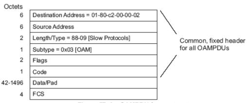
Figure 57–9—OAMPDU frame structure
