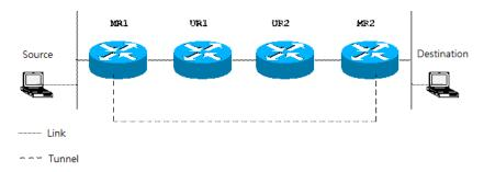
After the static multicast routing is configured, the router can perform the RPF check according to the configuration information. The RPF check is not based on the unicast routing table any more. Therefore, the multicast message goes through the tunnel, while the unicast message does not go through the tunnel. The static multicast route only exists in the local place. It will not be announced or forwarded.
