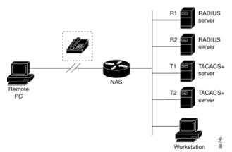
Figure 6-1 Typical AAA Network Configuration
