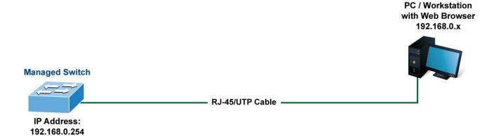
Figure3-6 Manage the Switch by Telnet
