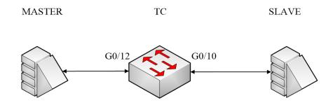
**MASTER** here stands for the master clock, which is a L2 PTP device. **SLAVE** here stands for the master clock, which is a L3 PTP device. TC stands for a switch that supports transparent clock. The master clock connects port g0/12 of the switch, while the slave clock connects port g0/10 of the switch. MASTER, TC and SLAVE are all working in P2P mode. Ports g0/10 and G0/12 belong to VLAN1.
