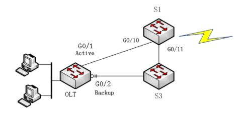
Figure 2: FlexLinkLite configuration example
