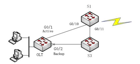
Figure 1: FlexLinkLite-enabled network
