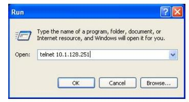
Figure 3-7 Run telnet client program included in Windows
