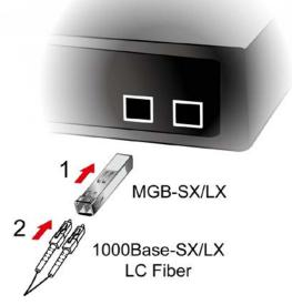
Figure 2-5 Plug in the SFP transceiver
