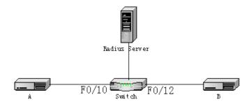
Host A connects port F0/10 of the switch. Host B connects port F0/12. The IP address of the radius-server host is 192.168.20.2. The key of radius is TST. Port F0/10 adopts remote radius authentication and user binding. Port F0/12 adopts local authentication of eap type, and Multi-hosts are enabled at Port F0/12.
