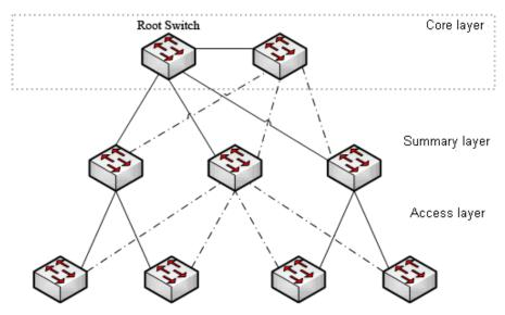
Figure 1.2 Switching network topology
