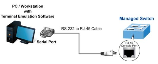
Figure 3-1 Out-of-Band Management Configuration Environment
