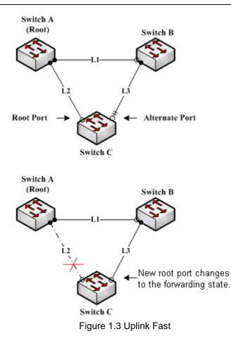
The Uplink Fast feature adjusts to the slowly convergent SSTP and PVST. In RSTP and MSTP mode, new root port can rapidly enter the Forwarding state without the Uplink Fast function.
