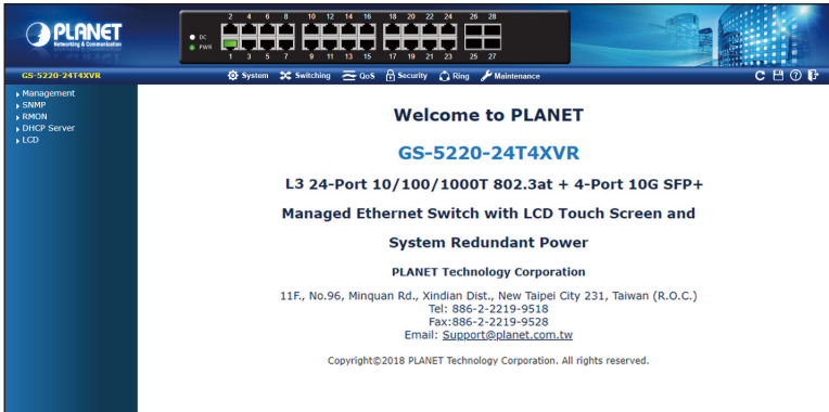
Figure 4-3: Web Main Screen of Managed Switch
