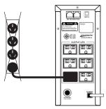
Enable the UPS by turning on the Power ON/OFF switch, which is situated on the front panel.
