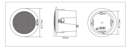
1. Drilling a hole, the size please refer to the dimension diagram.
